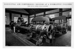
Horizontal air compressing engines at Normanton Collier. Graces Guide, from The Engineer 01/06/1911
